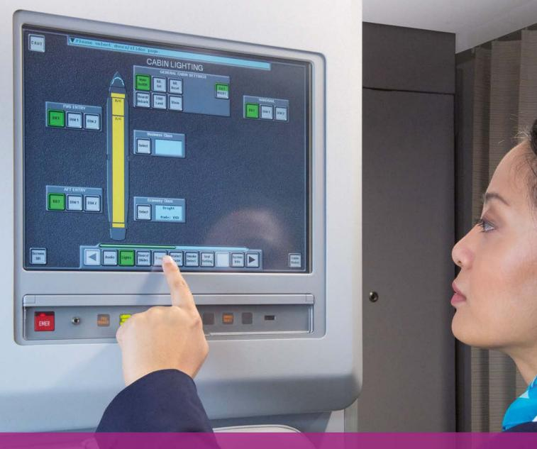
For all Airbus aircraft types, it is the CIDS (Cabin Intercommunication Data System) which is the key system for the aircraft cabin and enables management of cabin lighting, passenger service system functions, EVAC (evacuation) signals, cabin interphone and cabin system monitoring.
