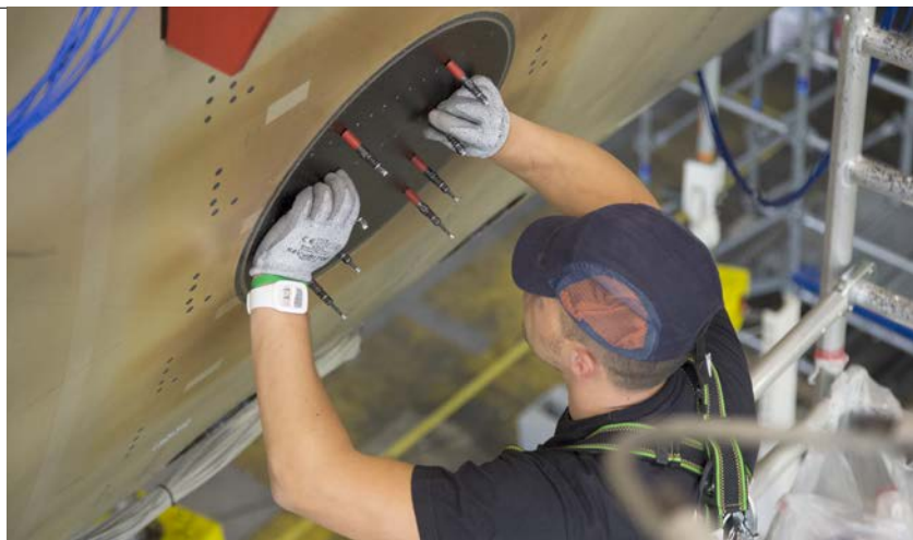
A complex repair, mixing bolted and bonded techniques
