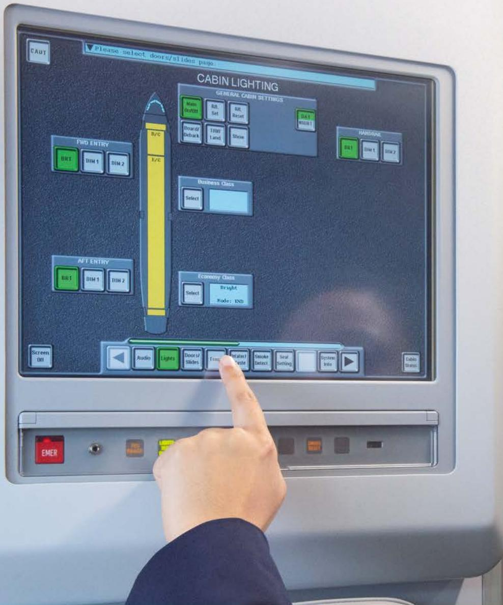
For all Airbus aircraft types, it is the CIDS (Cabin Intercommunication Data System) which is the key system for the aircraft cabin and enables management of cabin lighting, passenger service system functions, EVAC (evacuation) signals, cabin interphone and cabin system monitoring.
