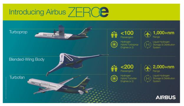
Other ideas we are looking at are extra-performing wings or totally new aircraft configurations like the "blended wing body" for a next generation, zero-emission aircraft. This new aircraft shape could bring fuel savings of up to 20% compared to current single-aisle models/configurations. Not only that, but the design could also open up new possibilities for different types of propulsion systems.
