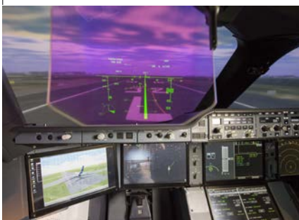
Head-Up Displays allow pilots to access relevant information in their direct line of sight
