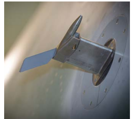
The increased rapidity of the sensors in the Multi-Function Probe enabled the Load Alleviation Function to be enhanced to facilitate increased design weights.
