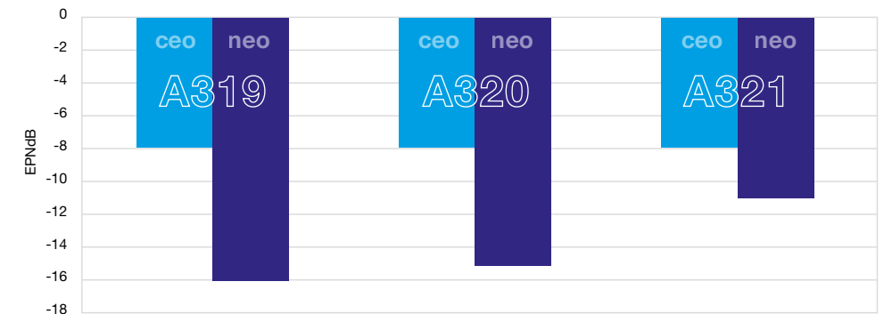
Reduced noise with the neo compared to the current A320 Family (excluding A318 aircraft) • Average of -4 EPNdB at take-off • Average of -2 EPNdB during approach
