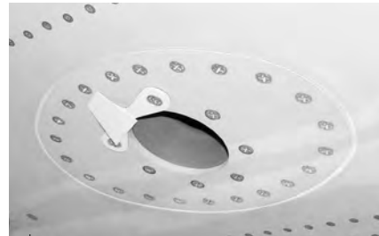
Underwing cavity fitted with air flow deflector
