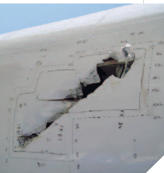
Damage on fuselage skin
