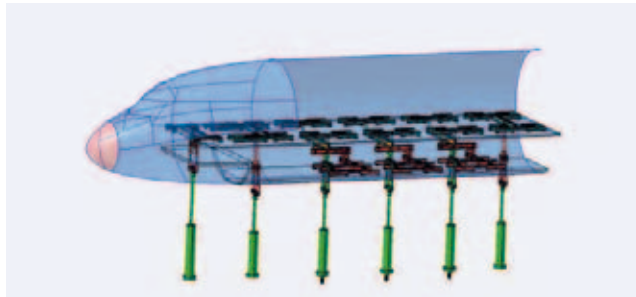
3D view of test facility environment to perform pylon fatigue test
