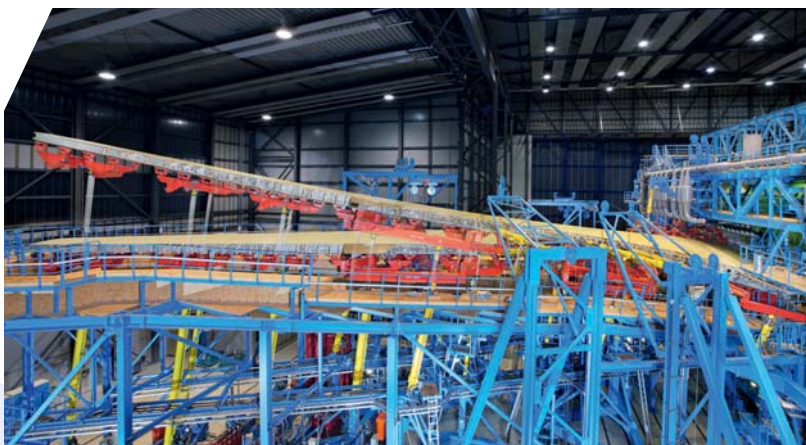
FSFT performed on each Airbus aircraft programme since 1970's - here for the A380
