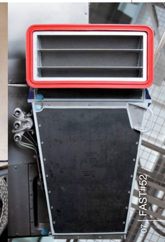
APU intake system
