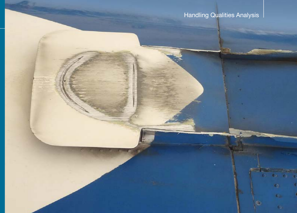
Damage on an Auxiliary Power Unit drain mast following a tail strike event
