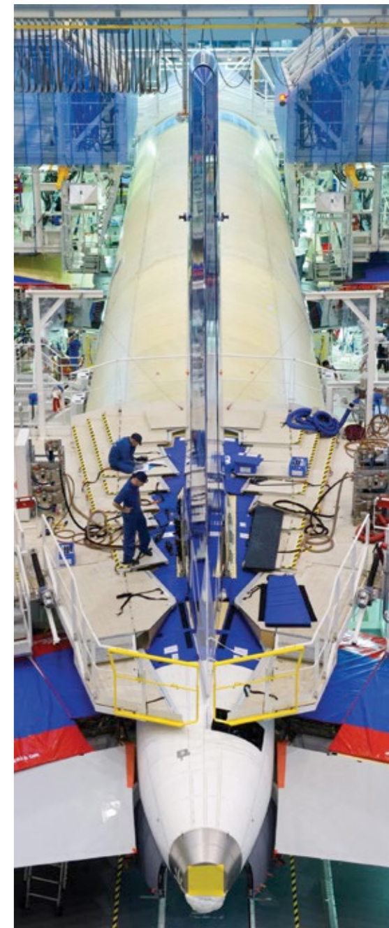
Installing the first A350 XWB tail
