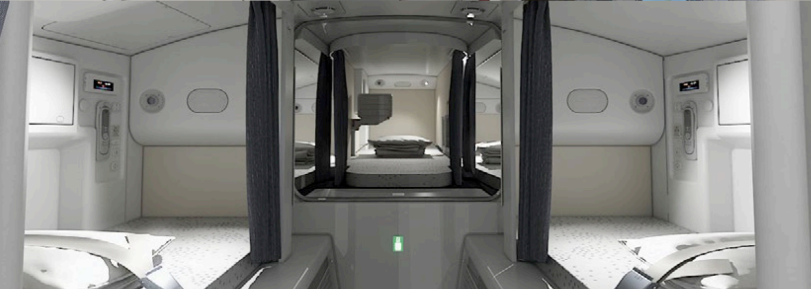
Flight crew rest facilities directly accessible from the cockpit with a secured entrance
