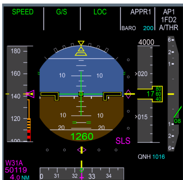
PFDD diagram showing closeup of horizontal and vertical guidance symbols.
