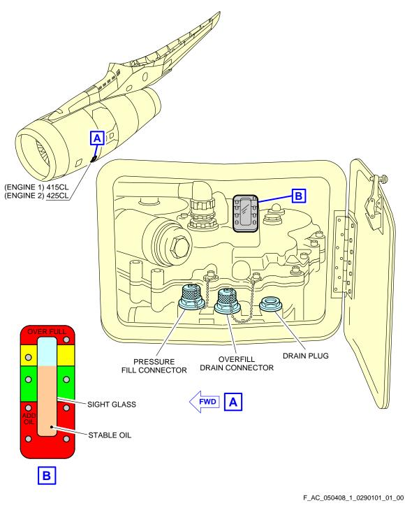
Ground Service Connections IDG Oil Tank - RR Trent 700 Series Engine FIGURE-5-4-8-991-029-A01
