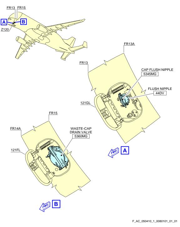
Ground Service Connections Waste-Water Ground-Service Panels FIGURE-5-4-10-991-008-A01
