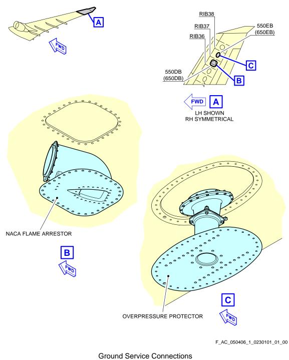
Overpressure Protector and NACA Flame Arrestor - Wing FIGURE-5-4-6-991-023-A01
