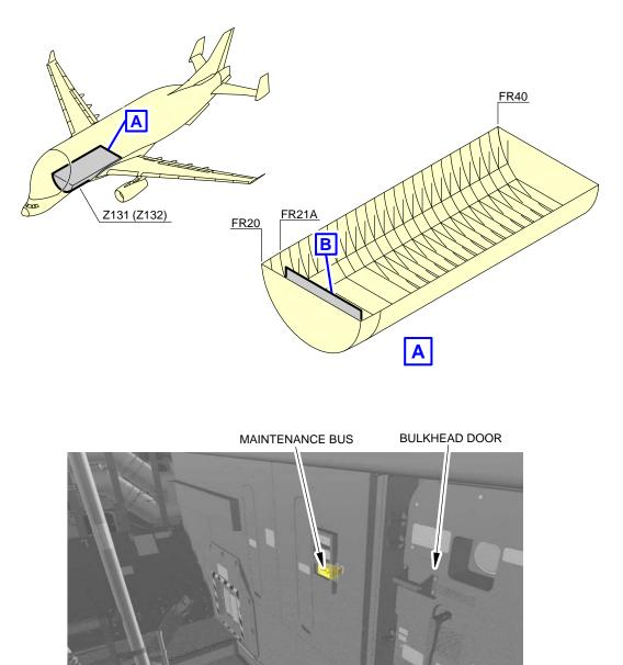
Ground Service Connections Maintenance Bus-Switch Location FIGURE-5-4-4-991-008-A01
