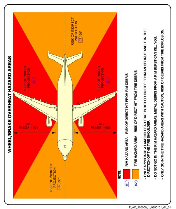
Wheel/Brake Overheat Wheel Safety Area (Sheet 1 of 2) FIGURE-10-0-0-991-089-A01
