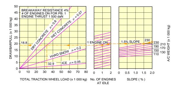
EXAMPLE HOW TO DETERMINE THE TRACTION WHEEL LOAD REQUIREMENT TO TOW A A330 AT 230 000 kg, AT 1.5% SLOPE, 1 ENGINE AT IDLE AND FOR WET TARMAC CONDITIONS:
