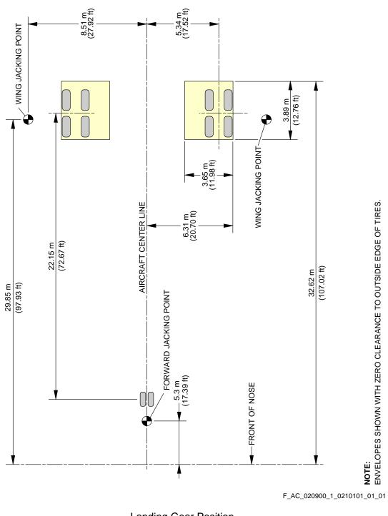
Landing Gear Position FIGURE-2-9-0-991-021-A01
