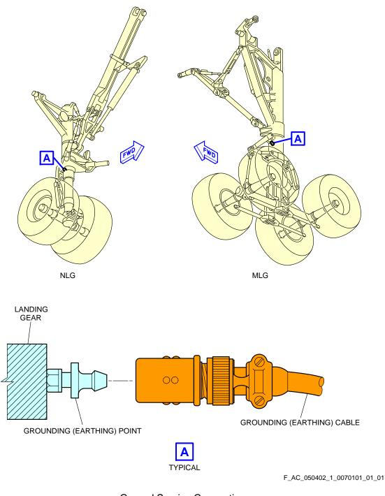
Ground Service Connections Grounding (Earthing) Points FIGURE-5-4-2-991-007-A01
